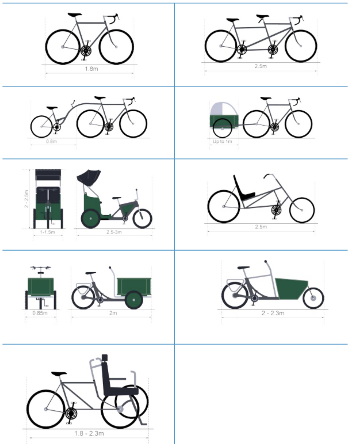
Figure 5.2: Typical dimensions of cycles
